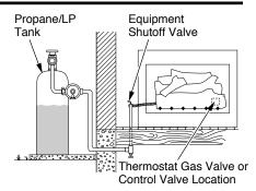
Figure 16 - Checking Gas Joints
